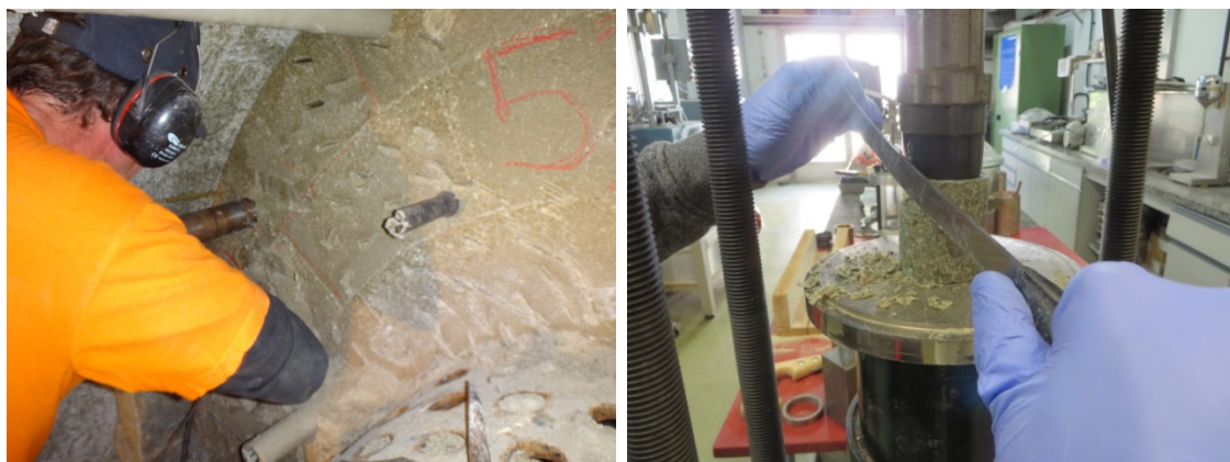
Fig. 121: Sample drilled on site at the contact between blocks (left), adjusting the diameter during sample preparation (right).
