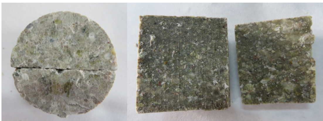
Fig. 123: Appearance of a specimen prepared for gas test with interface between blocks.
