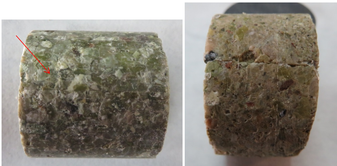
Fig. 122: Interface in a sample from the external ring (indicated by an arrow, BC-44-6) and from the inner ring (BC-44-2).
