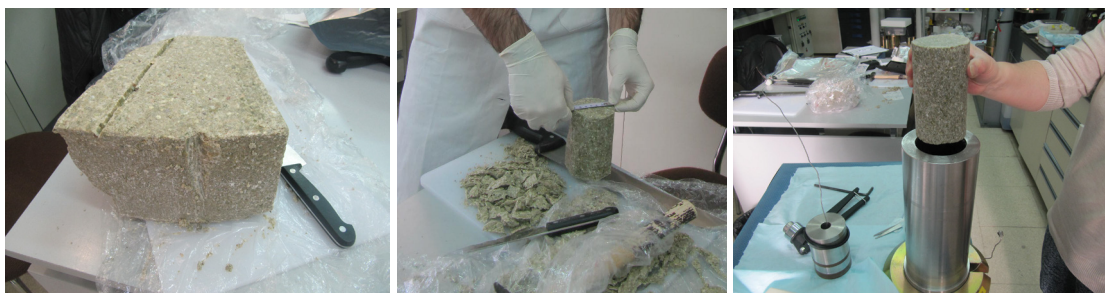
Fig. 85: Preparation of a sample for a squeezing test.
