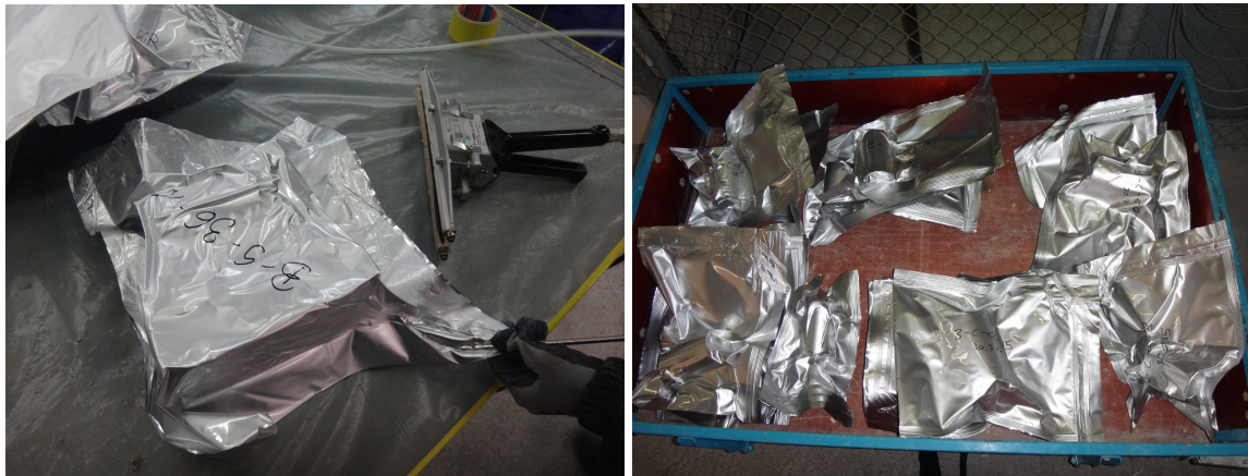
Fig. 5: Vacuum-packing of blocks at the GTS (left) and packed cores ready for shipment (right).
