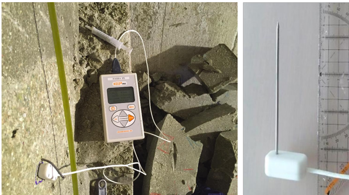
Fig. 88: Thermal analyser used by Nagra for the in-situ determinations during dismantling (the syringe contained the thermal grease) and needle sensor.
